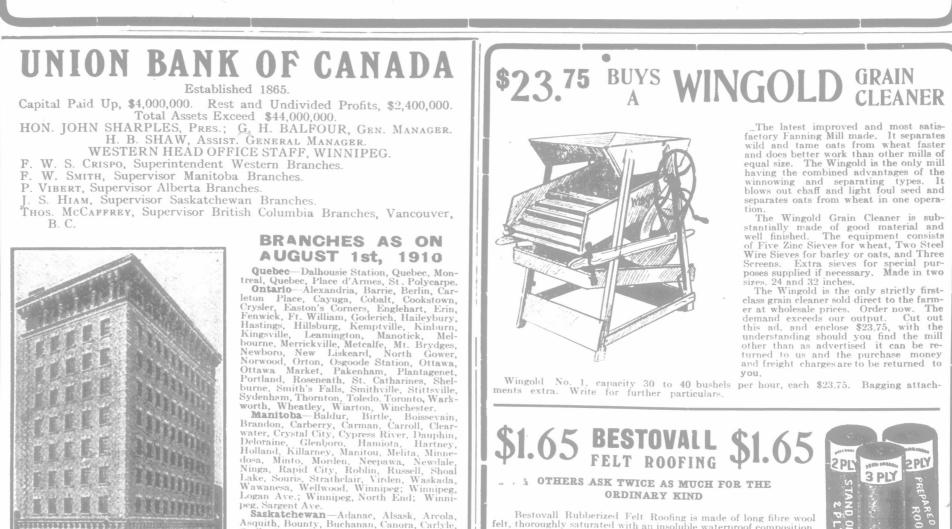
\_The latest improved and most satis-factory Fanning Mill made. It separates wild and tame oats from wheat faster and does better work than other mills of equal size. The Wingold is the only mill having the combined advantages of the winnowing and separating types. It blows out chaff and light foul seed and separates oats from wheat in one opera-tion.
