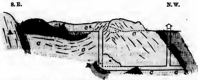
A, Hill limestone; B, underlying shale; C, cupriferous limestone; D, hanging shale; E, greenstone; C2, Dark coloured silicious limestone, distinctly stratified, with impregnating copper pyrites.
