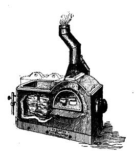
In case of a bullion spill the trap can be opened and the bottom removed without disturbing the brickwork of the furnace.
