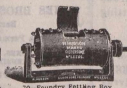
70—Foundry Fetting Box
