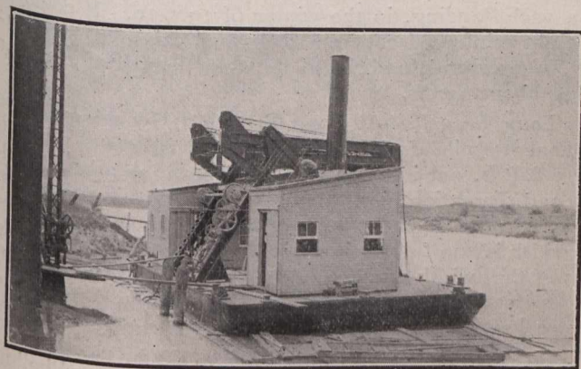
Fig. 2.—Gate Lifter with Top of Derrick Lowered for Passing Under Overhead Bridges.
