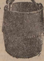
45—Mining Ribble with or without Valve in bottom
