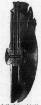
Sectional view of double-disk furrow opener, showing how the oil reaches the bearing and bearing construction. Note that the oil enters the bearing from the inside.
