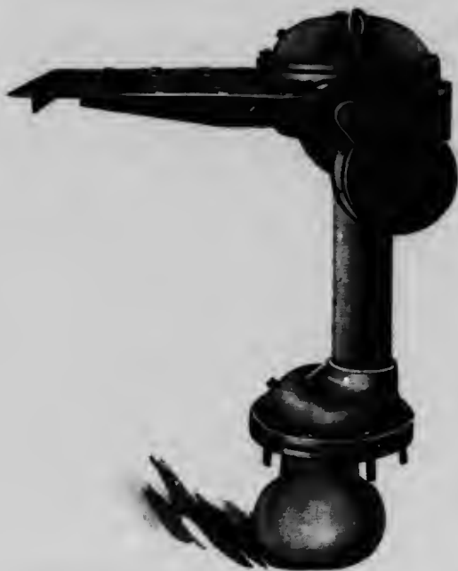
Submarine warning bell detached from bottom of buoy.
