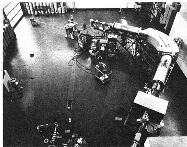
**THE TARGET AND THE CONTROL**—The particles fired by the gun end up at ground level (pictured above) in the target area. Experiments are performed on the beam of particles, with most of the action taking place in the control room (at right). The centre is known for its neutron time of flight and energy measurements, a feature not duplicated anywhere else in the world. All photos are courtesy the U of A Photographic Service.
