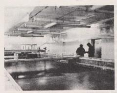
Various simulated Arctic ice conditions created at Arctec Canada's Kanata, Ontario laboratory enabled engineers to test the design for Polaris' dock facility.
