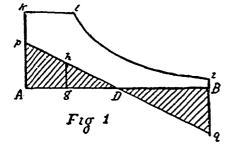
any point, g, in the left hand part of the horizontal base line, to the top line of the shaded part, gives the force exerted on the reciprocating parts in accelerating them at the corresponding piston position; and any similar line measured downward, in the latter part of the stroke, gives the effort exerted by these parts in being retarded.
