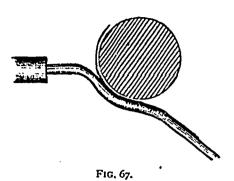
Quite a number of other e-periments might be mentioned, proving the same facts. The rotation of the ball is produced by the friction of the air currents passing over the ball, and is, therefore, a secondary result.
