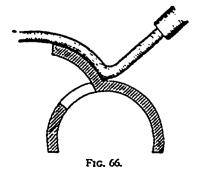
low the curvature of the surface until it meets a counter-current sufficiently strong to prevent a further rarefaction. If this view can be substantiated, it is plain that two external forces are acting upon the ball. One, the impact of the air current at  $\delta$ , transmitted at right angles to the surface, acts radially, and can be represented by the line  $\delta \beta$ . The other force,  $\delta q_0$  is
