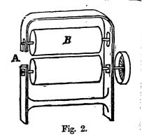
It is again weighed and the loss in stack a certained. The seed is taken off by mean cast iron rollers, (Fig. 2) making twelve reations per minute. They are solid, nineter inches in length and twelve in diameter. J handful of straw is taken by the operator r the seed end passed between the rollers at j the root end being, firmly held by the hand-This is repeated three or four times, and theby are sufficiently crushed. The roller B, is r to move upwards.
