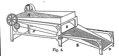
The chaff passes over to the floor at F. In gives motion to it, causing it to rise and hih a jerk. A horizontal motion is given by the crank-rod F, worked by the p nion Chas a motion similar to A. funcrushed bolls separated by the seive A,
