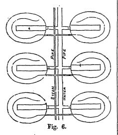
I will notice here, the method of Schenck. Fig. 6 is a ground plan of six vats, showing also, the steam pipe and water-pipe. Water is admitted by this pipe from a reservoir or tank on a higher level than the surface of the vats. This is heated by steam, to any required temperature.
