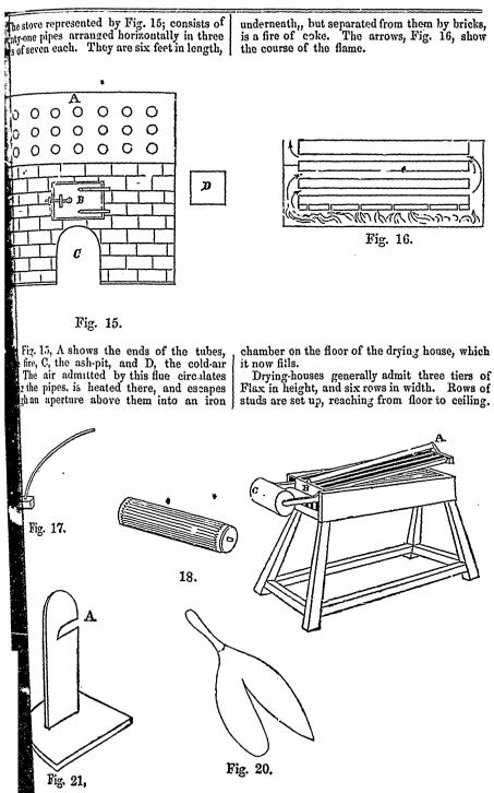
Horizontal bars are nailed to these in a longitudal direction, on which the holders are suspended. The apartments are air-tight above. The only means of escape for the air as it becomes charged with moisture, being by descent to spertures in the floor leading to shafts, and up these to ventilators in the roof.
