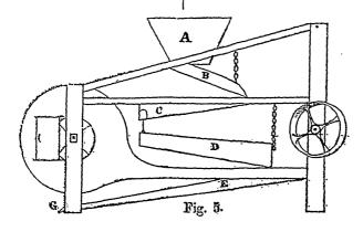
isside view of the fanners are represent | tal motion from cranks, and two serves (C, E) shuffle-boards (B, D;) having a horizon | moved by cams. The serve C is made of par 1
