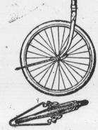
TO PREVENT ACCIDENTS the contact is head on the speed of the rear bicycle is checked, but if it is a trille to one side, as is usually the case, the fender causes the front wheel of the rear bicycle to glance off without causing a fall and injuring either rider. By actual tests it has been shown that with the use of this device collisions that would otherwise have upset the riders and entangled the machines, injuring both, have not even unseated the rear
