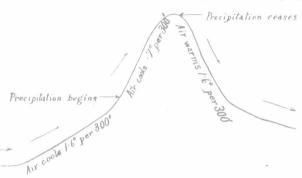
compression, almost instantly precipitation ceases and the rate of heating is 1.6 degrees for each 300 feet of descent. A diagram will enable us to understand the effect of these different rates.
