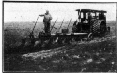
Case-Sattely 6 bottom 14 In. Automatic Lift Tractor Gang Plow—Gold Medal Winner in small plow class
