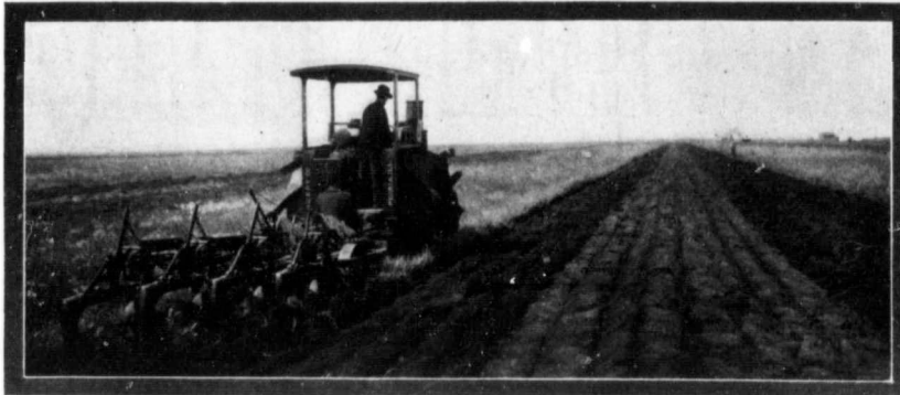
The Avery 12-25 H. P. Gasoline Tractor, Silver Medal Winner, Class A, Gasoline Engines; pulling an Avery 4 bottom power lift plow. Note the straightness of the furrow ridge, and the beautiful class of work done by this outfit. Do not be misled and think it is a two man outfit. The man sitting on the plow is the observer reading the Dynamometer.
