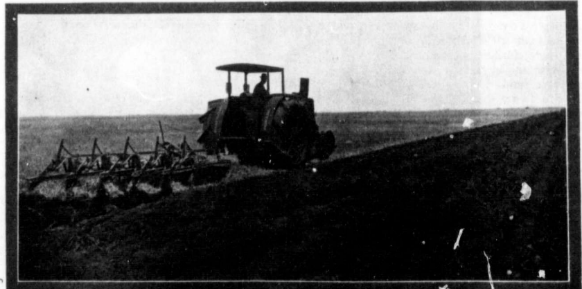
The Avery 20-35 H. P. Gas Tractor: Winner of the Silver Medal, Class B, Gasoline Engines; pulling a five bottom Avery Power Lift Plow, and doing a most excellent piece of work
