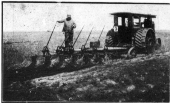
Pulling 6-14 in. Brake Bottom Plow—Average Draw-bar H. P. Gasoline 18.53 Average Draw-bar H. P. Kerosene 19.48
