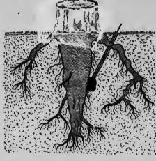
This picture shows the correct placing of the charge where the stump has a tap-root. The root will be broken off at sufficient depth to admit of the use of a plough.
