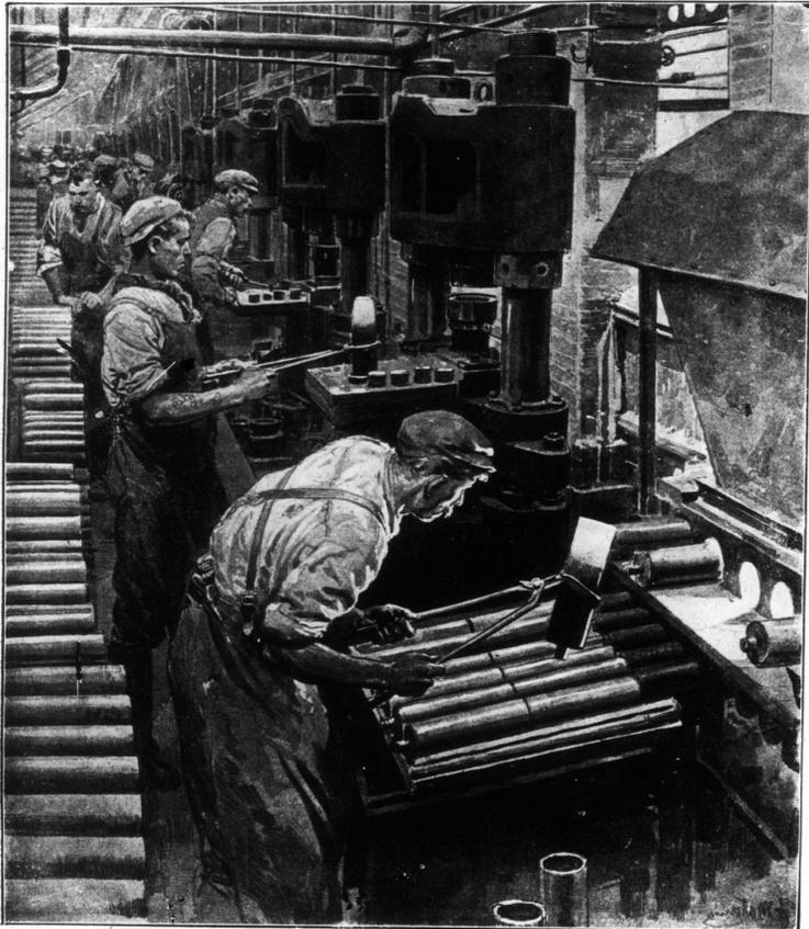
"Nosing" 18-pound shrapnel shells after heating in a British ammunition factory, operated by Vickers Limited. After being "nosed" and finished the shells are ready for the time fuse and charge. This drawing made by F. Matania, The Sunday World special artist from observations in the factory.
