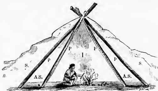
CROSS-SECTION THROUGH AYAN WINTER TENT. I., Interior; P. P. P. P., Poles; A.S., Air Space; S., Snow.
