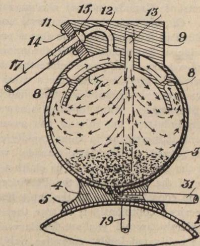
The apparatus is automatic in action, commencing to operate when the steam pressure in boiler reaches 10 lbs. Many of these cleaners are in active service and giving entire satisfaction. It can be attached to all kinds of boilers, and is especially adapted to those of the locomotive type.
