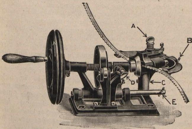
The amount of this movement is regulated according to the size of the saw tooth by the thumb screw. The file only cuts to a certain depth each time and this feature always insures accurate and even teeth.
