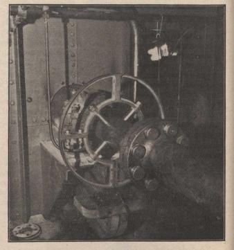
Angle-measuring Instrument on Shaft.
