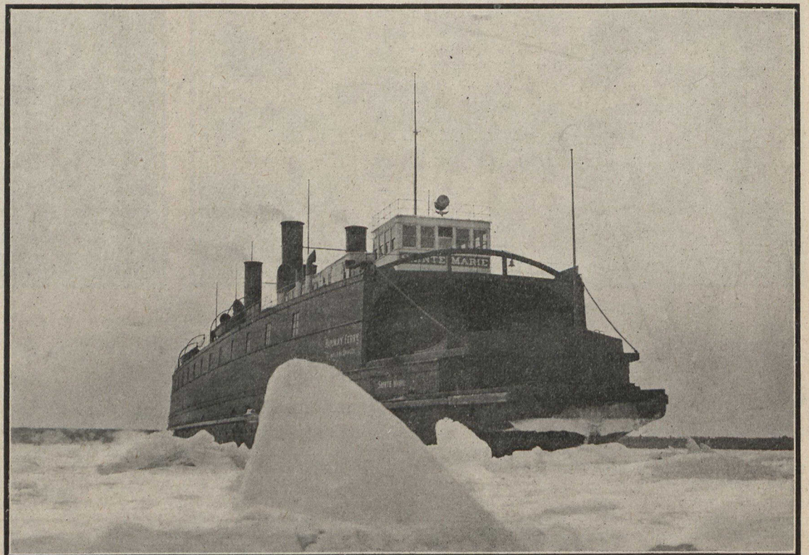
The "Saint Marie," an ice-breaking ferry which defies the effect of Winter upon the waters of Lake Michigan. The broken ice is sucked down in front and passes back through grooves under the vessel.
