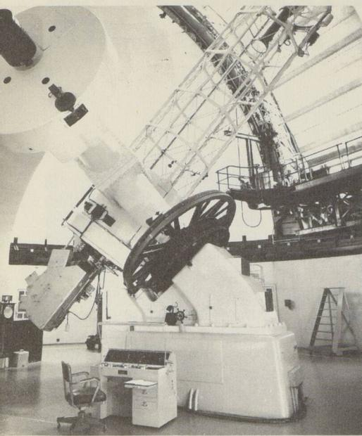
The mounting of the 72-inch reflecting telescope (above) at the Dominion Astrophysical Observatory, Victoria, B.C., permits it to be directed to almost any part of the sky. To follow a star, the telescope is driven by the clock mechanism just beneath the big wheel. Motors which move the 45-ton telescope are controlled from the movable console, foreground. The Observatory's 48-inch telescope (below) is equipped with modern, powerful spectrographs considered the most efficient in the world.
