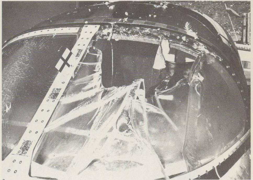
The compressed air gun is shown at left. At right is the shattered windscreen of a Tutor jet. Damage was done by an eight-pound chicken carcass travelling at 212 miles per hour.
