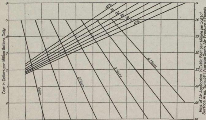
Fig. 2.—Cost of Activated Sludge Treatment for 50,000,000-gallon Plant.
