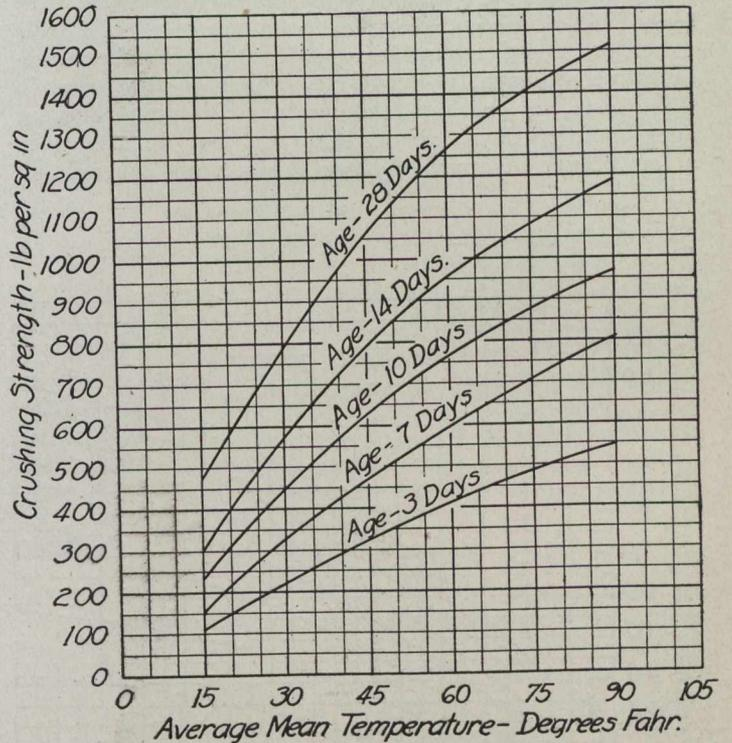
**Fig. 1.—Relation of Strength to Temperature for Different Ages.**
