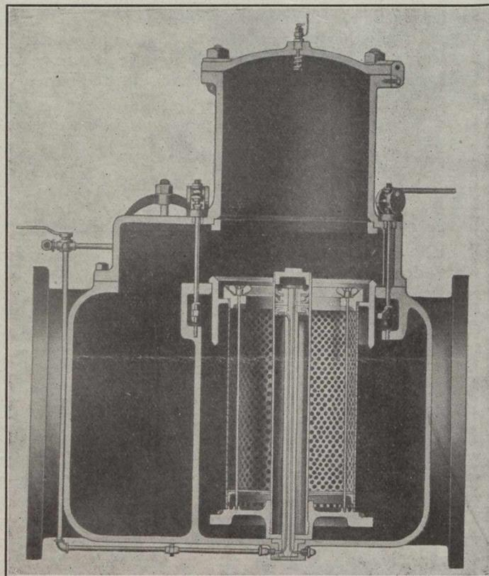
Fig. 2.—Section Through End Basket, Showing Cylinder and Control Valve.
