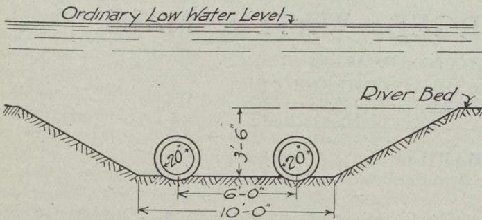
Fig. 2.—Trench Dredged in River Bed, for the Pipe Lines.
