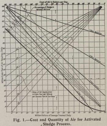
an example of the use of the diagram the arrows show the procedure for 50,000,000 gal. of sewage, 2 hours aeration, 0.25 cu. ft. per million rate of air application
