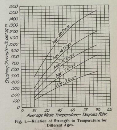
perature of the room and of the concrete, and the average time of molding.
