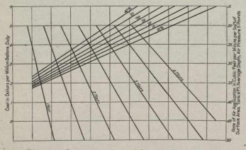
Fig. 2.—Cost of Activated Sludge Treatment for 50,000,000-gallon Plant.
