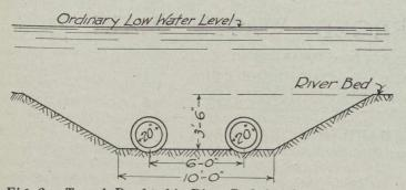
Fig. 2.—Trench Dredged in River Bed, for the !'ipe Lines.
