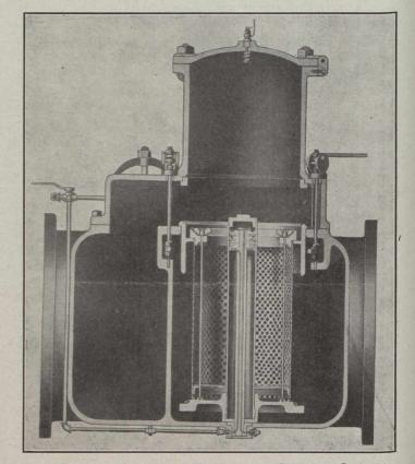
Fig. 2.—Section Through End Basket, Showing Cylinder and Control Valve.
