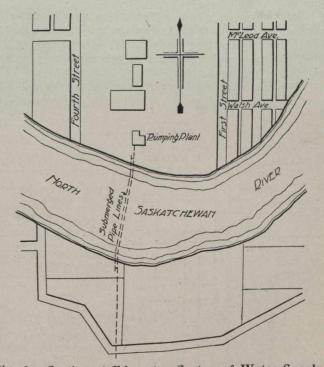
Fig. 1.—Section of Edmonton System of Water Supply, Showing Location of Two 20-inch C.I. Submerged Mains.
