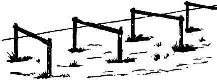
Fig. 51.—PLAN FOR EXACT GRADING.
