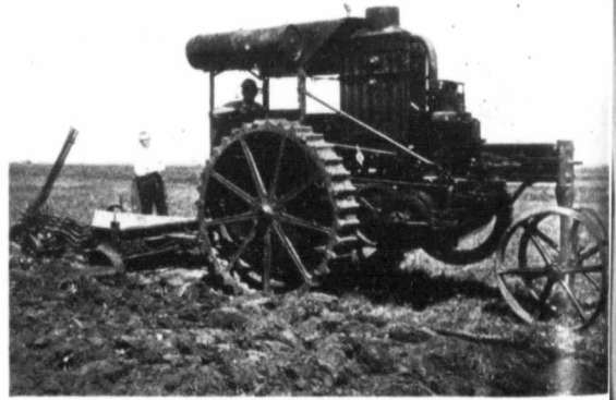
Hart-Parr 27 H.P. "Hopmaker" Tractor burning Kerosene and pulling a 4-bottom Powerlift Hart-Parr Engine Gang
