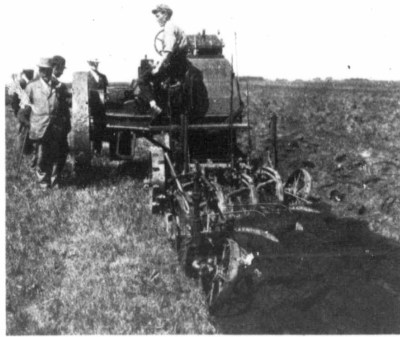
The Grain Growers Special 12-24 Light Tractor pulling a 4-bottom, Lacrosse Self-Lift Plow
