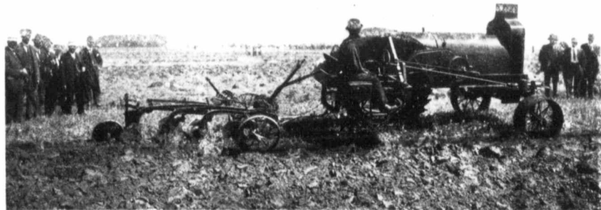
Hart-Parr 22 H. P. "Little Devil" Tractor pulling a 3-furrow Cockshutt Special Light Tractor Fiv
