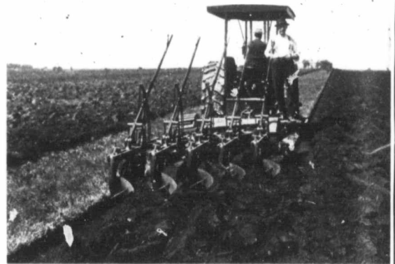
Sawyer-Massey 16-32 Kerosene burning Tractor, pulling a 5-bottom 14-inch Powerlift Cockshutt Engine Plow
