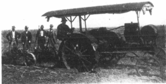
"Waterloo Boy" 12-24 Light Tractor burning Kerosene and pulling a John Deere No. 3 Pony 3-furrow Engine Gang
