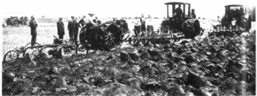
The Canadian Avery String Avery Self-Lift Plows were pulled in each case. See specification tables for sizes
