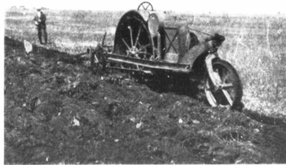
7-20 Canadian Bull Tractor Pulling a 2-furrow Powerlift "Enicar" made by J. I. Carr Plow Works, Racine, Wis.
