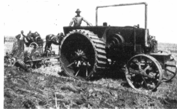
Gold, Shapley & Muir 15-25 "Ideal" Kerosene Tractor, pulling a 6-bottom Cockshutt Powerlift Engine Gang
