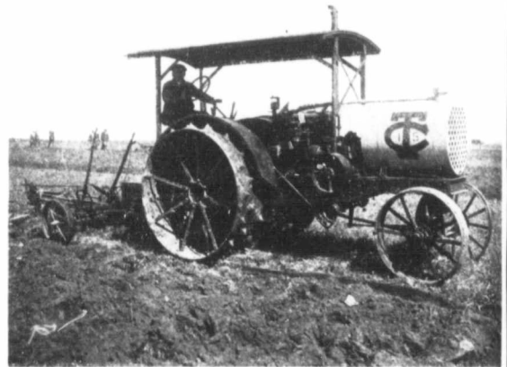
"Twin City" 15-30 Kerosene Tractor Pulling a 3-furrow John Deere No. 3 Pony Tractor Plow Equipped with Deere Detachable Shares and a Powerlift
