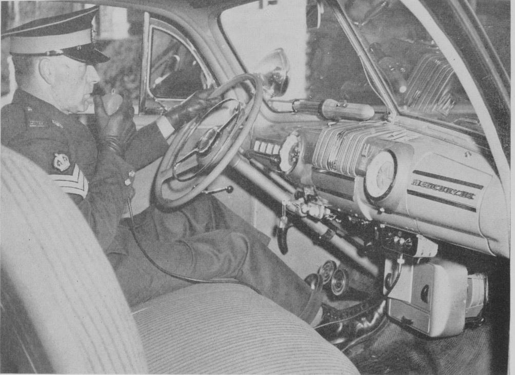
*Above:* Interior view of patrol car showing part of the two-way radio installation.
