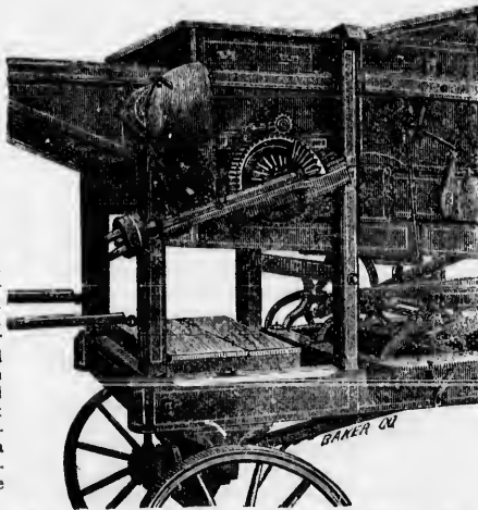
Section of "Grain Saver" showing Side Gear, Crank Shaft & Tool Box.
