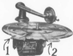
Motor Mechanism and Metal Motor Board No. 1 indicates speed-regulator and start and stop lever. No. 2 shows speedometer.
