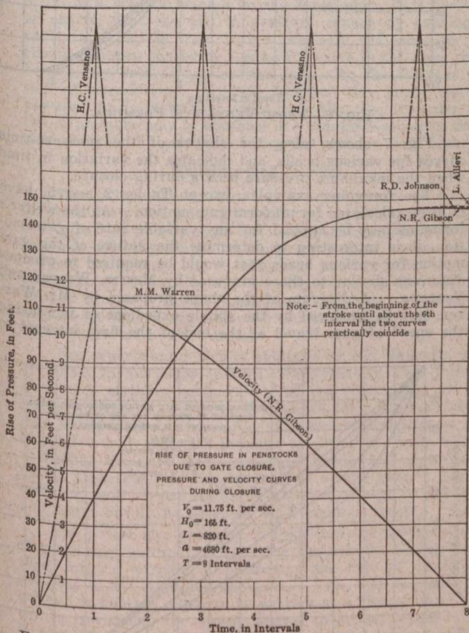
FIG. 5—PRESSURE AND VELOCITY CURVES DURING CLOSURE
