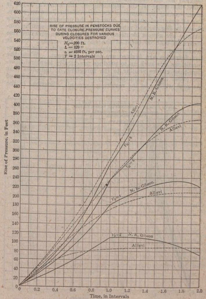
FIG. 6—PRESSURE CURVES DURING CLOSURES FOR VARIOUS VELOCITIES DESTROYED
