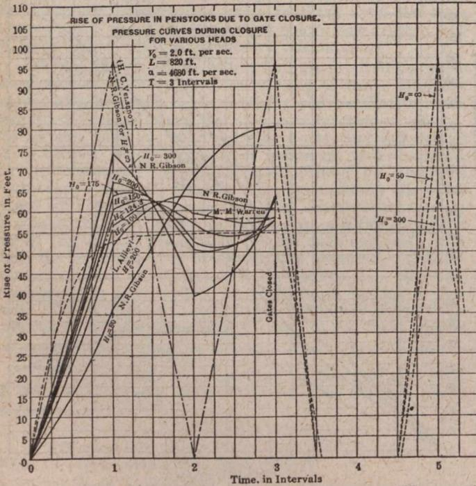
FIG. 7—PRESSURE CURVES DURING CLOSURE FOR VARIOUS HEADS
