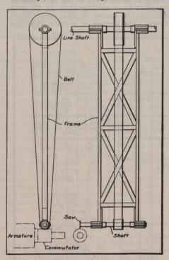
Rig for Slotting Commutators to Remove Mica.
