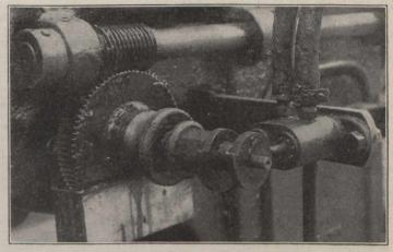
Fig. 6 .- Automatic Chucking Mechanism.
