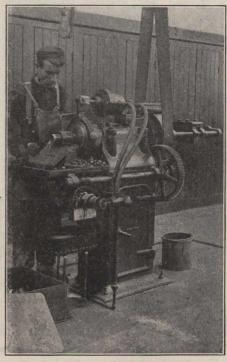
Fig. 4.-Automatic Safe-end Machine.
