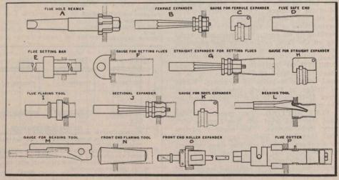
Fig. 31.-Tools Used in Preparation of Flue Sheet.
