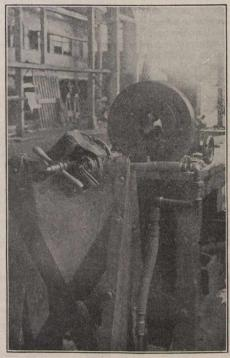
Motor Operated Pipe Threading Macnine.
