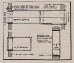
Fig. 28.-Method of Setting Flues in Flue Sheet.
