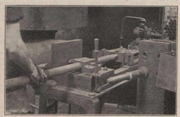
Fig. 3.--Flaring the Cut-off End.
