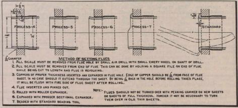
Fig. 29.-Method of Setting Flues in Flue Sheet.
