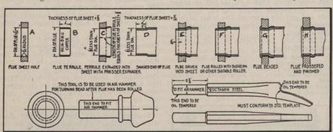
Fig. 30 .- Method of Setting Flues in Flue Sheet.
