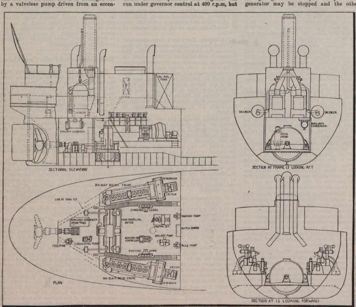
Arrangement of Machinery in Diesel-Engined Ship with Electric Drive for the Montreal Transportation Co.
