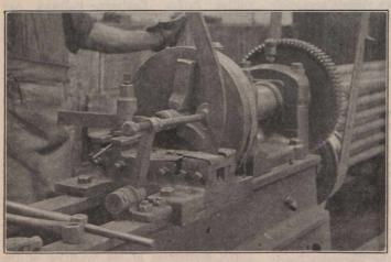
Fig. 2.-Cutting off First Bad End.
