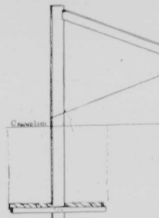
THE ANCHORING AND CORNER POST IS OF BUILDING. THE DRAWING METHOD OF DOING THIS, FEET 6 INCHES IN THE MATERIAL, NOTCHED IN POST BRACED IN THIS STRAIN OF 60 RODS OF FE NARI
