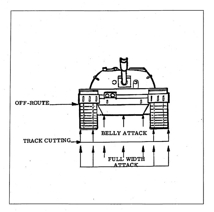
FIGURE 30 - TRACK, BELLY OFF-ROUTE AND FULL WIDTH ATTACKS
