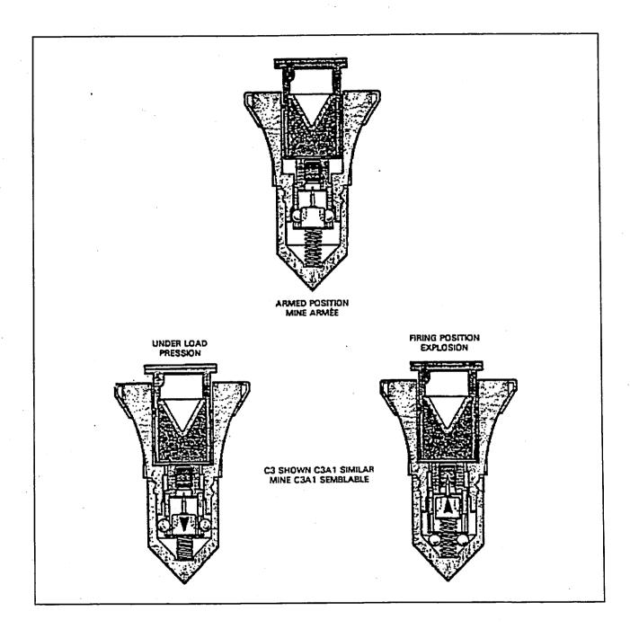
FIGURE 5 - FUNCTIONING OF ANTI-PERSONNEL MINE C3 AND C3A1
