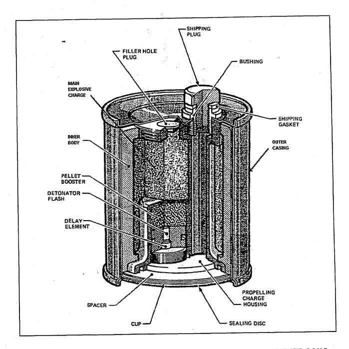
FIGURE 9 - ANTI-PERSONNEL MINE M16A2 SHOWN WITHOUT FUSE, M605
