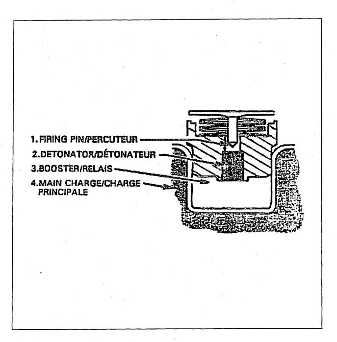
FIGURE 14 - GENERAL EXPLOSIVE TRAIN FOR ANTI-TANK MINE
