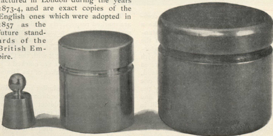
TROY OUNCE AND AVOIRDUPOIS POUND OF PLATINO-IRIDIUM, AND AIRY BRONZE POUND OF 1844. (ALMOST NATURAL SIZE)
