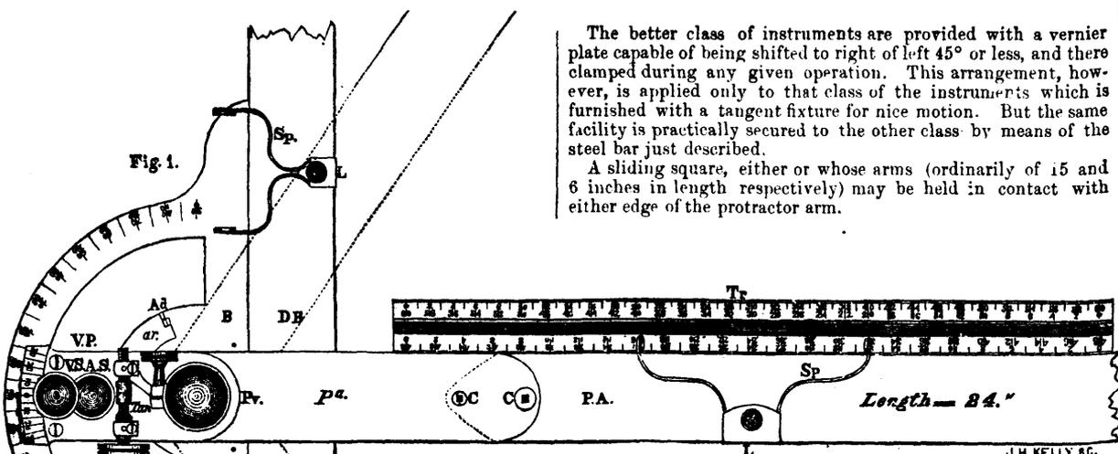
The better class of instruments are provided with a vernier plate capable of being shifted to right or left 45° or less, and there clamped during any given operation. This arrangement, however, is applied only to that class of the instruments which is furnished with a tangent fixture for nice motion. But the same facility is practically secured to the other class by means of the steel bar just described.
