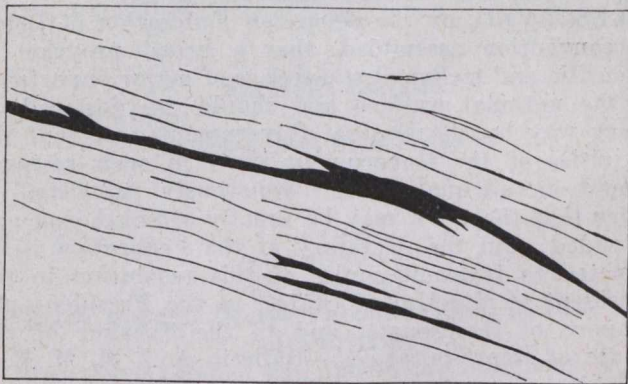
Sketch showing quartz veins at Howey-Cochenour-Willans gold prospect, Holloway township; east walls at depth of 35 feet in shaft. The length of vein system in sketch is about six feet. The main quartz vein is shown by the heavy black part; parallel stringers of quartz occur on each side of the main vein.—Bureau of Mines.
