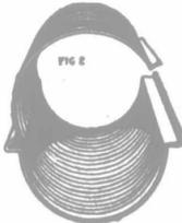
ribs, engage easily, as you see in Fig. 2. The joints between one length and another are "broken"—no over-lap reaches more than half-way round the culvert's diameter; and this is possible with NO OTHER metal culvert made. It is a most valuable feature, for it reduces the chance of leakage to the very least minimum.
