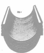
When the sections of Pedlar Culvert, of any diameter—it's made from 8 inches to 6 feet—reach you, they are nested like Fig. 1. Note the two distinct flanges—the radial and the recurved. These fit into each other, and are FLAT, while the CURVE of the culvert is corrugated. Place section on top of section, and the flanges, or locking-
