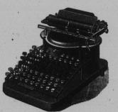
The New Yost No. 2. This machine is intended for experts where the greatest speed is required. Has the automatic type bar lock, by which the type is locked at the end of every line and prevents one letter being printed over the other. Also the new one motion line spacer in addition to all improvements on No. 1.
