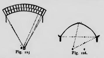
ing it. The joints for brick or stone work may be laid out around this arch, by using the centers as fixed points and running radial lines through the curved lines.
