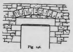
Another style of work is shown at Fig. 146, where the walls are formed of square stones laid
