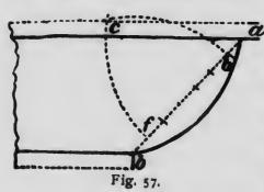
parallel to a, a; from b, with b, a, draw the semicircle b, d, and from d, draw to e, perpendicular to b, d; produce a, a, to e; from e, as a center,
