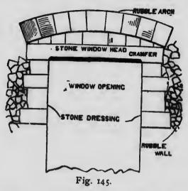
weight over to the jambs. The face of the window is all of dressed stone, while the walls are formed of irregular stones.
