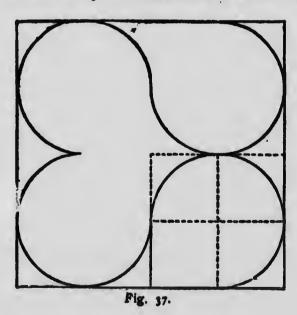
curves are drawn with one radius. The manner of getting the centers is shown by the dotted lines. Figs. 38 and 39 exhibit another combination of curves which is easy to draw. To make Fig. 39 is perhaps the easiest of them all, as it is formed of curves drawn with one point of the
