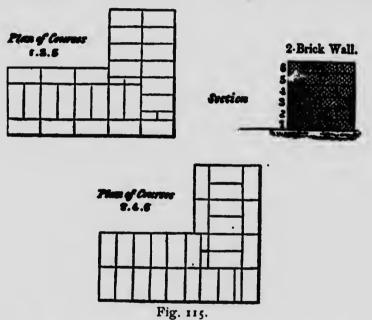
or stones placed in juxtaposition so as to prevent the vertical or plumb joint between any two bricks or stones falling into a continuous straight line with that between any other two. This is called "breaking joint," and when it is not properly carried out, that is, when two or more joints do fall into the same line, as at x y,
