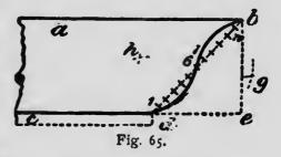
g, with 8 as a center, and the same radius, describe the arc 67b, then with 1 and 6 as centers describe the arcs at h, with h as a center, describe the arc d, 6.
