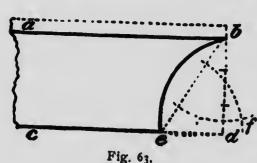
mould. To describe it let ab, cd, Fig. 63, be the lines at top and bottom. From b, draw to d, perpendicular to a, b; divide bd,
