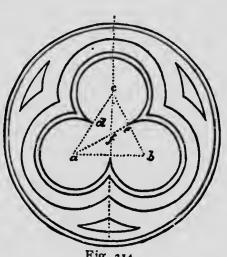
foil ornament, as used in windows and other decoration, and is formed as follows: Draw the equilateral triangle as shown by the dotted lines a b c, then bisect it as at c f and a e, cutting the line c f, which gives the center for the surrounding circles; a b and c are the centers of the trefoil curves.
