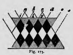
shaped pattern. The dotted lines show the construction, the distance between the diamond as e f g h, a b c d, being equal to the distance a f, a d e. The use of
