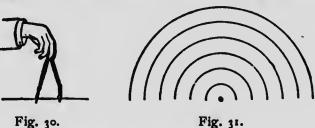
thickness of lines, and the pen should always stand vertically over the work, as shown in Fig. 30. When a number of circles drawn from a common center is necessary, as shown in Fig. 31, be sure to draw the outside, or the one having
