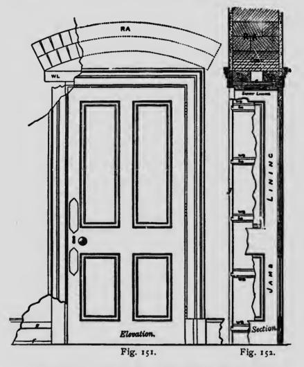
The jamb linings go right through the depth of the opening, and on one side of the wall have their edges rebated to receive the door; the
