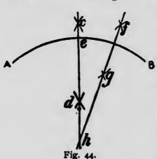
pass through the center. Then from points e and b, with a rather shorter radius, strike arcs intersecting at f and g, draw a line through these intersections. and where the previous line is cut will
