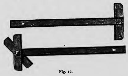
of the stocks having ebony or other hard wood glued on the edges to prevent them from wearing. The lower square has a movable stock, which is operated by a thumb screw, thus enabling the draftsman to set the blade to any angle desired. The working of this will be easily understood by the reader.
