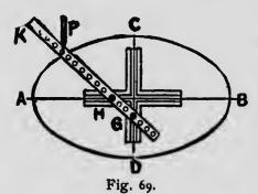
very simple. The instrument consists of two principal parts, the fixed part in the form of a cross as C D, A B, and the movable tracer H G. The fixed piece is
