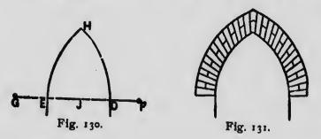
arch. This is drawn by placing the centers of the curves outside the figure as at G and F. E. O, show the width of the opening, and H J, the height.
