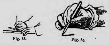
Fig. 88 shows the T-square and pencil with the two hands in position for drawing an ordinary horizontal line. The pencil should be upright when looking in the lengthways direction of the line, and sloping about five degrees from the upright in the direction in which it is being drawn, as would be seen at right angles to the line, and in Fig. 89 the method of holding the pencil for freehand or tracing work is shown. This is on a larger scale in order to show the
