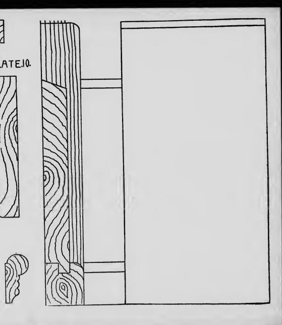
in its place on the wall. A section of a box window frame is shown at Fig. 164. The weights are seen in the box, the stud forming part of the box. This is designed for a balloon frame house, and it will be seen that the inside trim
