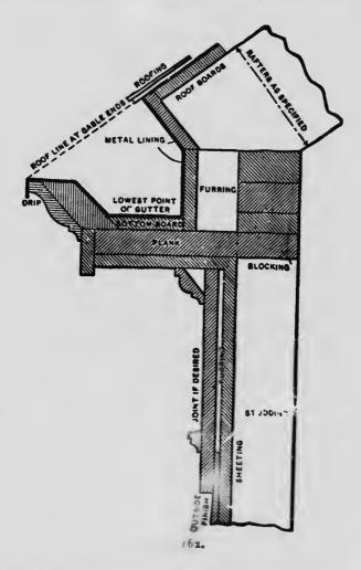
plete finish for cornice re shown; also, an iron rod or anchor built int the wall, having a nut on the top which is interested to hold the plate
