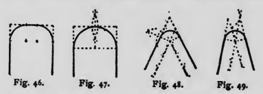
which the required circle is drawn. Determine the extreme position of the curve and mark from it, along the center line, a distance equal to half the distance between the lines, and this mark
