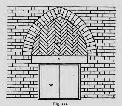
styles of laying bricks; C shows the arch A, herring bone filling over a window, S, a stone sill, F the general brickwork and W the window opening. This is a good example to draw, though it is not by any means good architecture.
