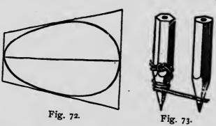
either pierces the string or the string is looped to hold the pencil, near the other pencil, which leaves the arrangement ready for work. To draw the scroll the pencils must be kept vertical, the point of the first kept firmly in the hole or center of the figure, and the second pencil must then be carried around the first, with the marking point held in touch with the paper, the distance between the two increasing regularly as the string unwinds.
