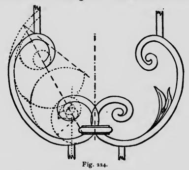
which the curves of the pattern are drawn. The method of forming scrolls has been described in a previous chapter, so that it is unnecessary to repeat at this stage. The design is simple, the centers being all given and the dotted lines show the radii of the curves.
