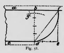
figure. Divide b, d, into four equal parts; make d, e, equal three of these; draw e, f; then with any radius greater than half of d, f, with d, and f as centers respectively,
