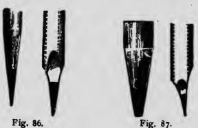
draftsman's hands. As before stated, all drawings of any importance should first be made in pencil; and a hard pencil should be used for the purpose; in fact, there should be two pencils, one of which should be pointed similar to those shown at Fig. 86, and the other should be sharpened with a chisel-point similar to those shown at Fig. 87. These two illustrations, Figs. 86 and 87, show two methods of sharpening, either of which will answer the purpose quite well.
