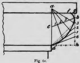
produce the line to c. Then from a, as a center, with the radius a, c, or a, g, describe the curve c, g. Fig. 60 is a method where the tangent d, e,
