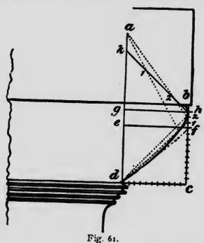
of equal parts, and through the points of division in e, b, draw from a, straight lines, and through the points of division in e, b, draw from d, right lines, cutting those drawn from a. The intersections will be the points through which the curve is traced.
