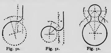
curve. In every case it will be observed that the perpendicular line from the center of the junction curve to the line, or the line joining the centers of the two curves, will give the exact termination of the junction curve.
