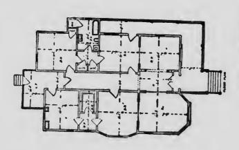
SIZE: Width, 40 feet Length, 72 feet Blue prints consist of cellar and foundation plan; roof plan; floor plan; front and side elevations. Complete typewritten specifications with each set of plans.
