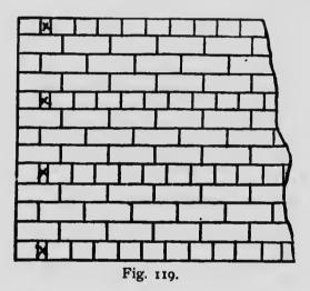
Thus, an English bond nine-inch wall will have for each course of stretchers two rows side by side, breaking joint horizontally. The joints in the inside courses should be one-half the width of the brick from the vertical joints of the stretchers above and below. A fourteen inch wall in English bond is shown at Fig. 120, which represents four courses in elevation, and the
