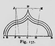
A B be the outside width of the arch, and C D the height, and let A E be the breadth of the rib.
