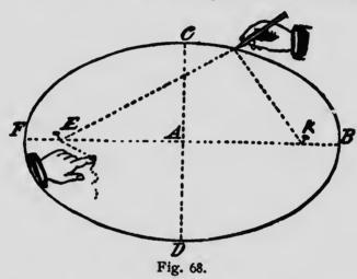
the pencil at C and run the string round it and carry the string to the pin E, holding it tight and winding it once or twice round the pin, and then holding the string with the finger. Run the pencil around, keeping the loop of the string on the pencil, and it will guide the latter in the formation of the curve as shown. When one-half of the ellipse is formed, the string may be used for the other half, commencing the curve at F or B, as the case may be. This is commonly
