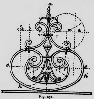
space between them equal to the space at c, as 1, 1, and with a radius equal to the diameter of these circles, describe from the points I, I, the arcs m, n; m. n. From n, n, which are equidistant from the center line, a space equal to the radius of the small circles n, p; describe with radius of these small circles the arcs meeting in the point
