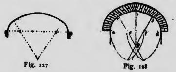
Tudor arch. It is struck from three centers as shown. It is sometimes called an elliptical Gothic arch, and may be struck as follows:
