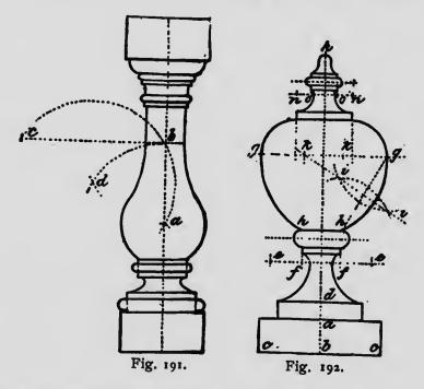
a describe an arc cutting the line c d in c; c in the center of the curve which is continued to the dotted line c b; a straight line is then continued to the neck of the baluster. The other curves and lines are readily obtained.
