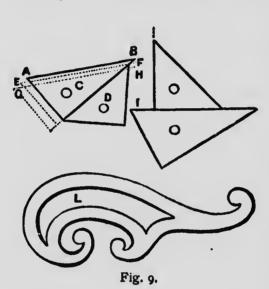
handy for drawing curves not easily struck by the compasses, and also for eccentric curves, which the compasses are not able to describe as in medieval mouldings of some forms. In in king-in a
