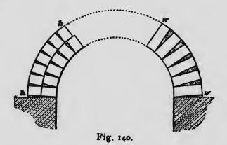
the mortar joints in this are much wider at the top than those of the portion hh, built in rings half a brick in thickness. The line of joints in both these examples are radial, all being drawn from the center point.
