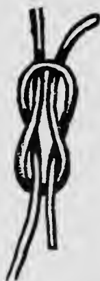
Reef knot or square knot: never slips or jams: easily loosed.
