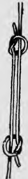
The fisherman's knot. It never slips; is easily opened by pulling the two short ends.
