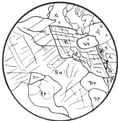
FIGURE 8.—Idiomorphic Hornblende Crystal in the streaked Syenite-gneiss.
