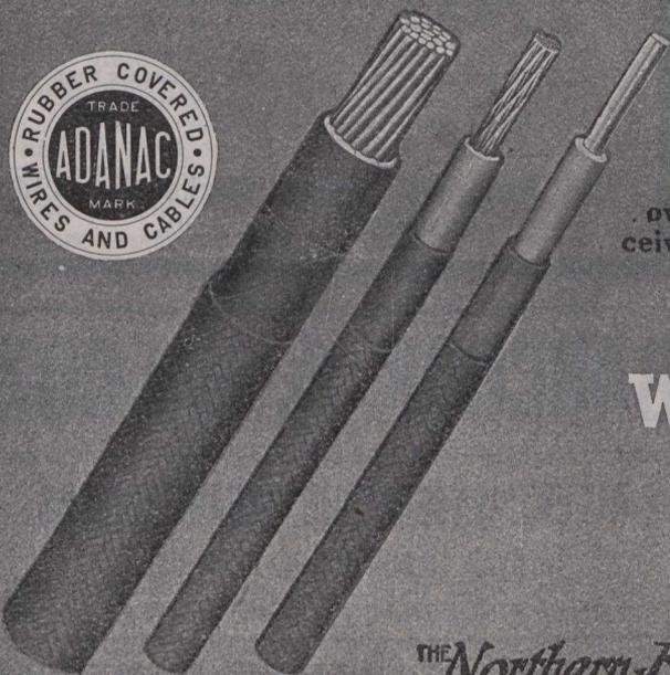
Are made according to the specifications of the National Board of Fire Underwriters. The conductors are drawn from copper of the highest conductivity and are covered with two thicknesses of thoroughly vulcanized rubber compound of high quality. The wires are braided over insulation and the smooth high finish they receive makes them specially desirable for conduit work.
