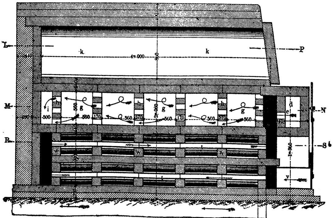
Fig. 2.—Longitudinal Section through Muffle.—Shown by A B, Fig. 4.
