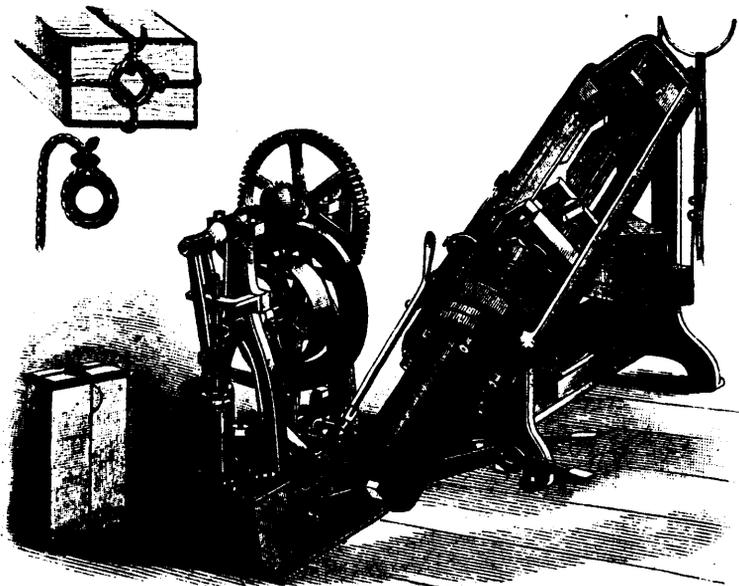
MACHINE FOR PRESSING AND PACKING PRINTED SHEETS.
