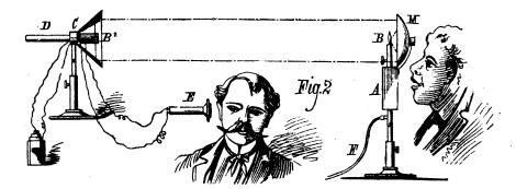
MAGNETIC THERMOPHONE WITH MANOMETRIC FLAME TRANSMITTER.
