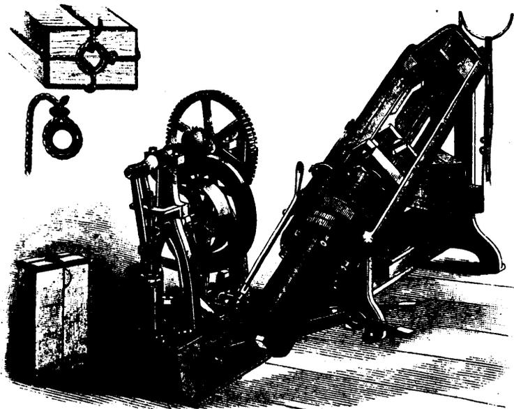
MACHINE FOR PRESSING AND PACKING PRINTED SHEETS.
