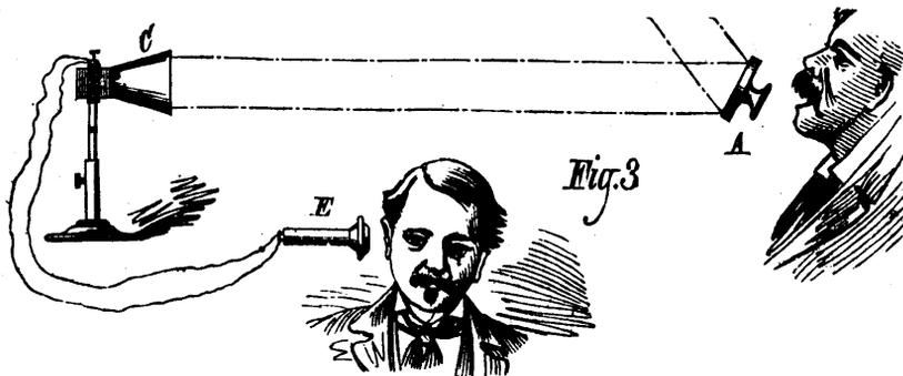
THERMOPHONE WITH THERMO-ELECTRIC RECEIVER AND REFLECTING DIAPHRAGM TRANSMITTER.
