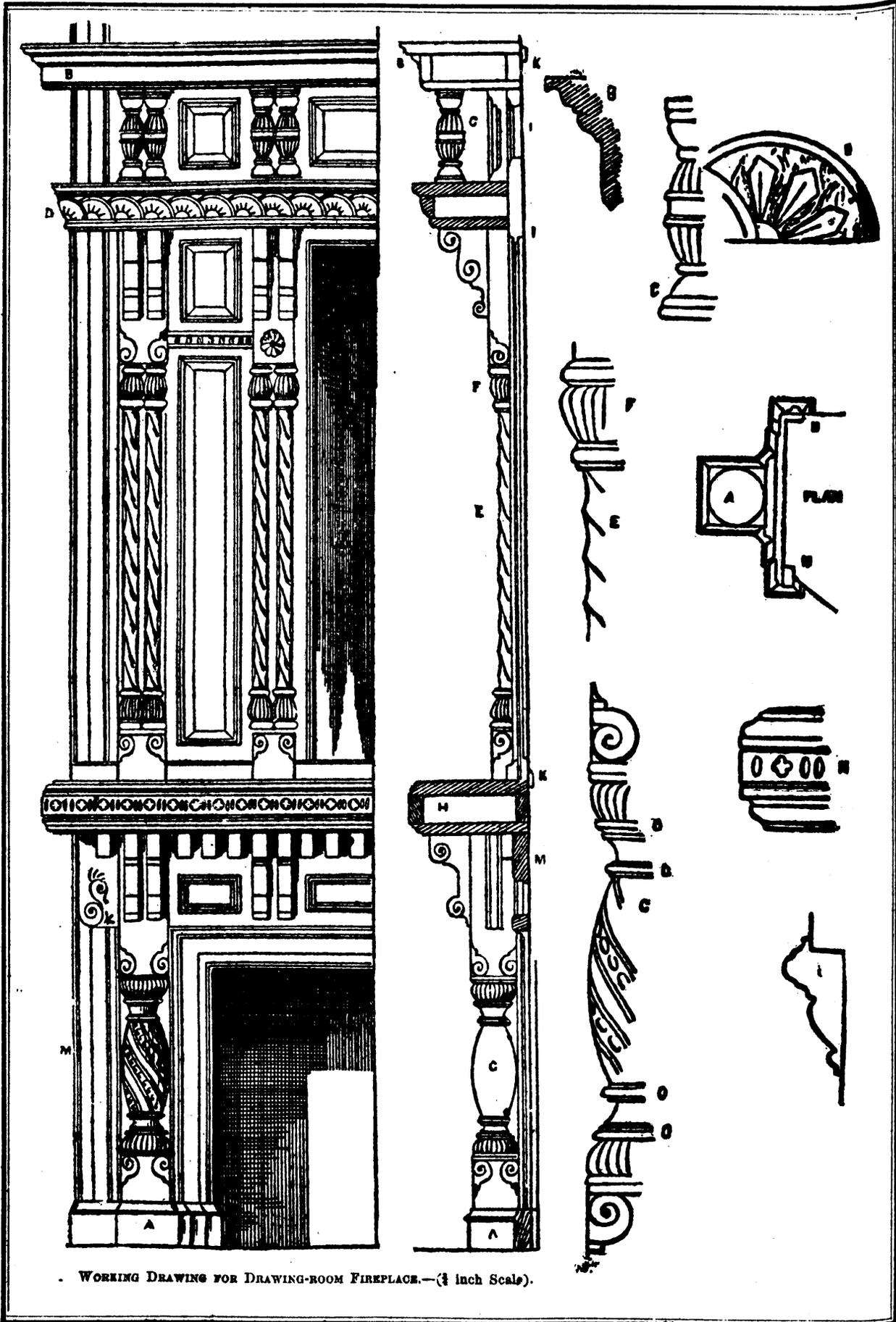
WORKING DRAWING FOR DRAWING-ROOM FIREPLACE.—( $\frac{1}{4}$  inch Scale).
