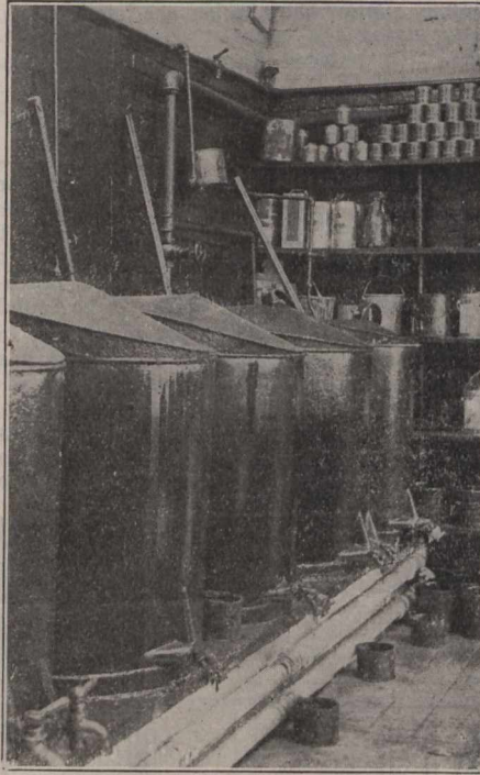
Fig. 3.—Paint Mixing Tanks.
