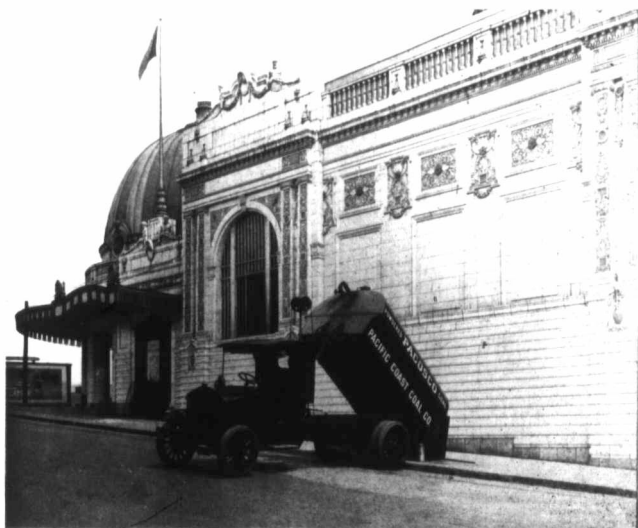
DELIVERING PULVERIZED COAL BY TANK MOTOR TRUCK The Crystal Pool, or Natatorium, Seattle, Wash.
