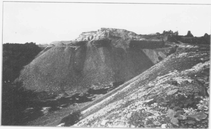
General view of quarry of bituminous sand-rock, operated by the City Street Improvement Co., near Santa Cruz, Cal. Average thickness bituminous sand-rock 60 feet. Overburden, hard shales 40-60 feet in thickness. Shipments from this quarry for year ending April 31, 1913, were 32,853 tons.
