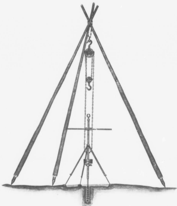
Fig 4. Arrangement of auger for boring Bituminous Sand
