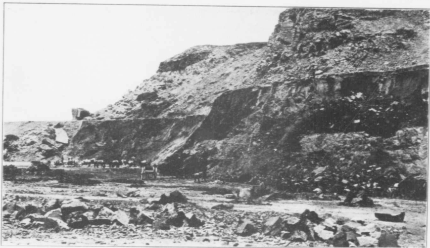
Typical quarry of bituminous sand-rock operated by City Street Improvement Co., near Santa Cruz, Cal., U.S.A. Average thickness of bituminous rock about 60 feet. Overburden consists of hard, Monterey shales, 40-60 feet in thickness.
