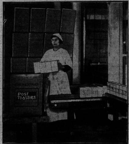
Scene in the Canadian Postum Cereal Company's Factory, Windsor, Ont. Sealed packages of Post Toasties emerging from packing machine at the rate of fifty per minute.
