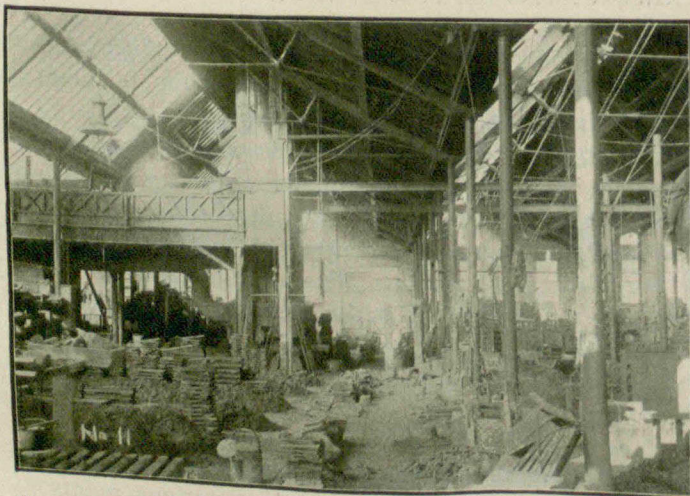
FIG. 3.—INTERIOR VIEW OF FOUNDRY, SHOWING CUPOLA AND CHARGING PLATFORM.
